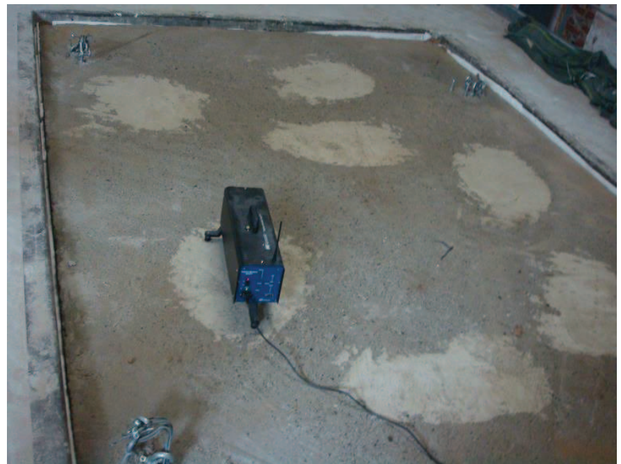
installed test setup with prefab screed slab during test
